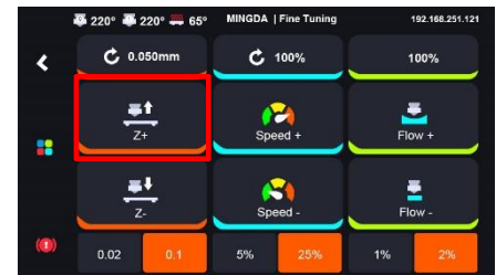
Select the distance at 0.02 and increase the Z-offset until the line is smooth
